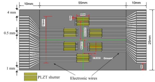
Fig. 6. Mask of six PLZT shutters.
