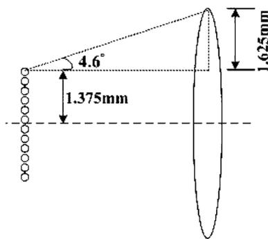
Fig. 8. Edge channel position of an input fiber ribbon.
