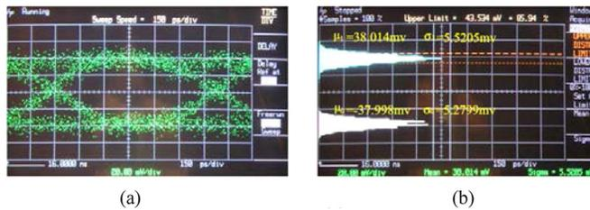
Fig. 13. Microsecond switching performance at GbE link. (a) Eye diagram. (b) Histogram.
