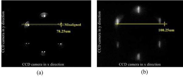
Fig. 12. Analysis of spot alignment error. (a) Misaligned spots on the L3 focus plane. (b) Misaligned spots on the SLM.
