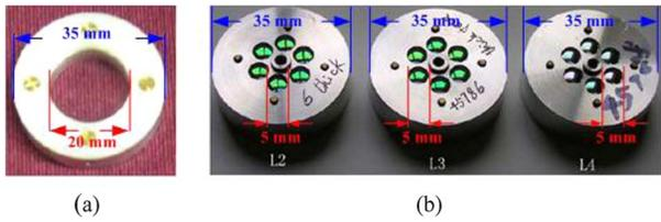
Fig. 3. Components of the optical fan-out subsystem. (a) Grating element. (b) Lens arrays held by custom-designed lens holders.
