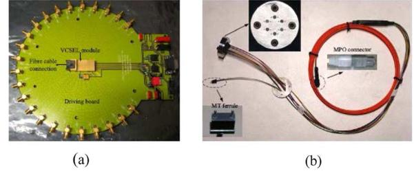
Fig. 2. VCSEL transmitter and input fiber ribbons. (a) ZARLINK VCSEL transmitter module and the driving board. (b) Six input fiber ribbons terminated with MT type connectors.
