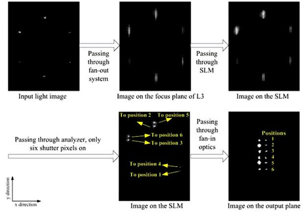
Fig. 11. Spot patterns on the key planes of a fiber ribbon switch.
