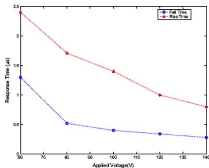
Fig. 7. PLZT response time and applied voltage.
