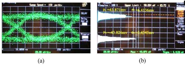
Fig. 14. Submicrosecond switching performance at GbE link. (a) Eye diagram. (b) Histogram.
