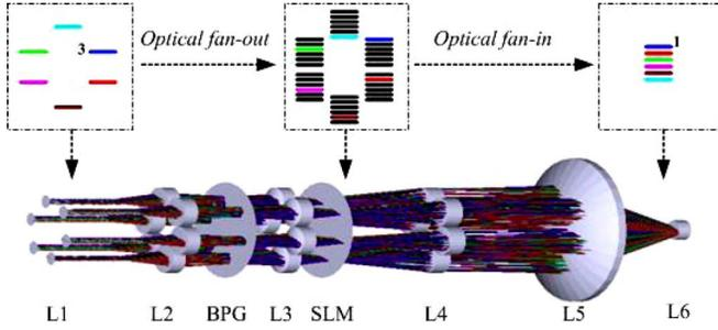
Fig. 1. Architecture and operating principle of the  $6 \times 6$  fiber ribbon switch.
