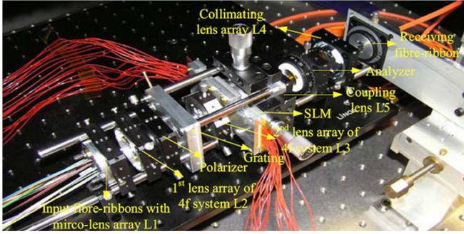
Fig. 10. Demonstrator of 6 × 6 72-channel optical fiber ribbon switch.
