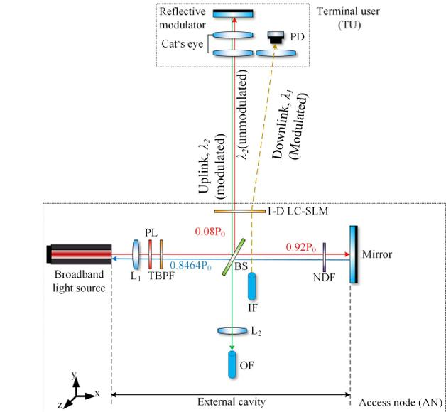
Fig. 1. System configuration of asymmetrical SIL-based B-OWC system.
