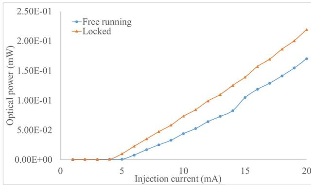
Fig. 3. Optical power & injection current under free running and SIL.
