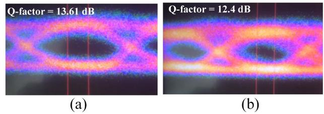
Fig. 4. Eye diagrams of uplink (a) 2 Gbits/s, (b) 2.5 Gbit/s. (at AN).
