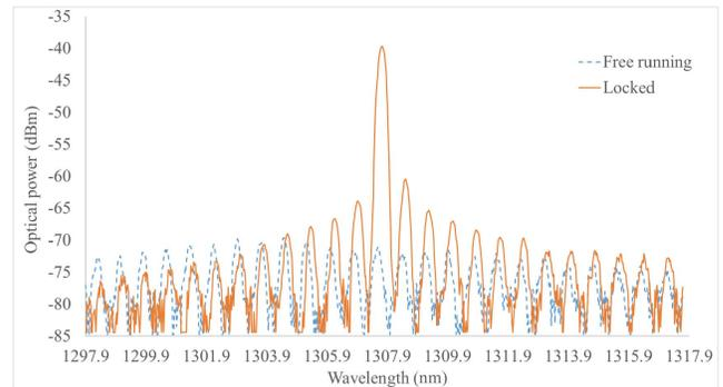
Fig. 2. Optical spectrum under free running and SIL. (at TU).
