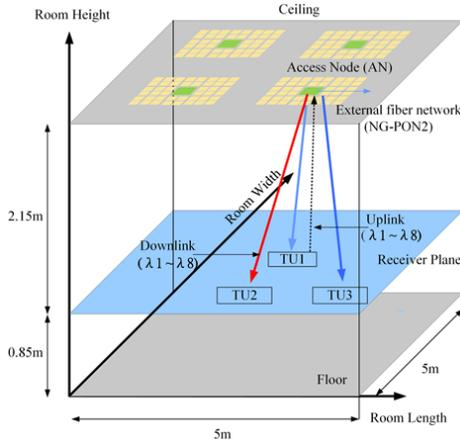
Fig. 1. LCoS-based access node in home area network
