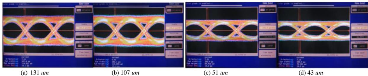
Fig. 5. Eye diagrams taken when the spot size focused at TU in downlink was expanded from  $43 \text{ um}$  to  $131 \text{ um}$  ( $\lambda = 1550 \text{ nm}$ )
