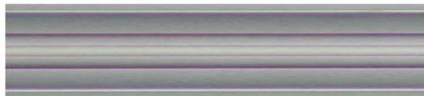
Fig.2. Photo of a double-clad Cr:YAG crystal fiber
