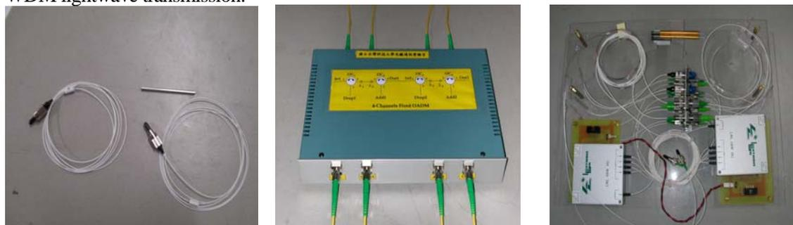
Figs. Temperature compensated fiber Bragg grating (left). Four-channel fixed WADM (mid.), and four-channel reconfigurable WADM.
